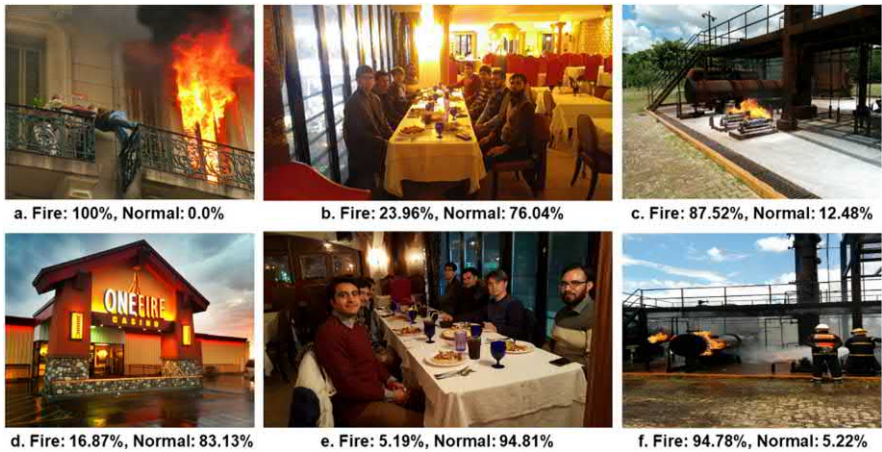
FIGURE 3.4 Sample query images along with their probabilities for CNN-based fire detection [7].
