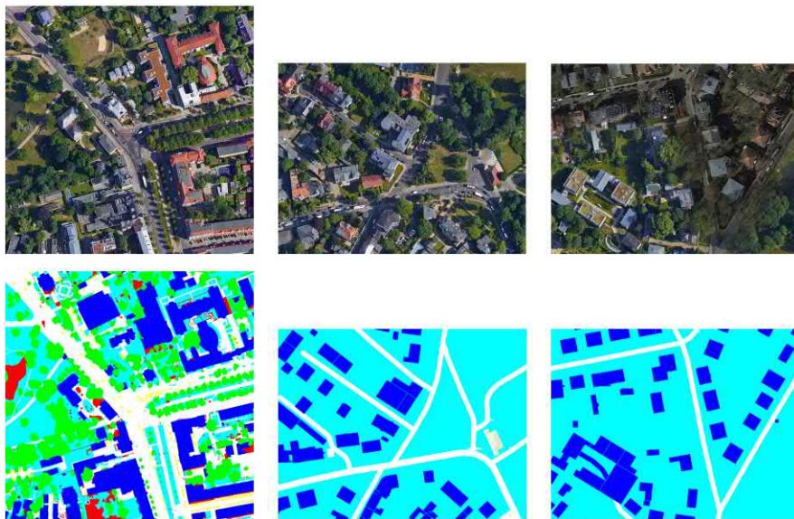
FIGURE 7.14 A sample of the Potsdam Extended dataset. On the top row, the left panel is the corresponding Google Satellite Image copying ISPRS’s tile and using its ground-truth. The middle and right panels are tiles produced from other areas in Potsdam. The bottom row is OSM as the ground-truth.
