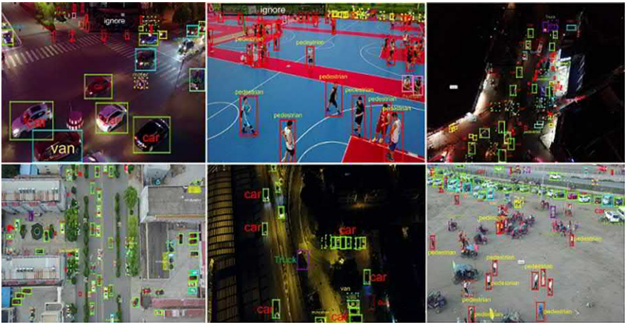
FIGURE 2.6 Six sample images from the VisDrone-DET2018 dataset. They are pictures taken from drones. The rectangular boxes on each image are ground truth. It has a large number of small objects at distance.
