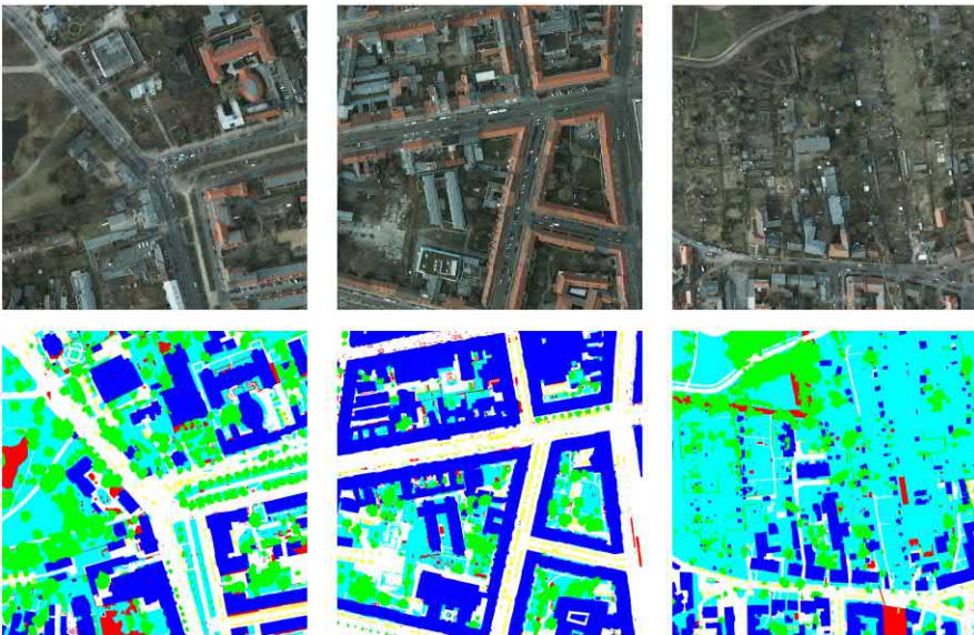
FIGURE 7.13 A sample of the tiles available from the ISPRS Potsdam 2D Semantic Labeling Challenge.
