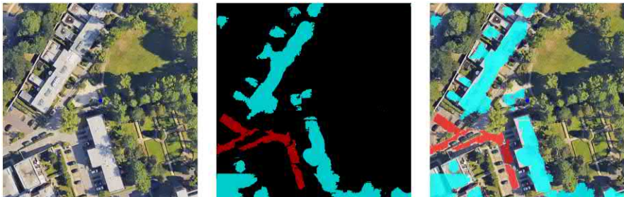
FIGURE 7.7 Buildings segmented using U-Net (the left panel is an EO image, in the middle panel is the result of segmentation, and the right panel is an EO image overlaid with segmentation).
