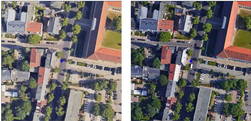
FIGURE 7.18 The left panel is S_n , and the right panel is the estimated r . The actual UAV GPS coordinate is \{52.404758, 13.053362\} , while the estimated GPS coordinate is \{52.404737, 13.053338\} .
