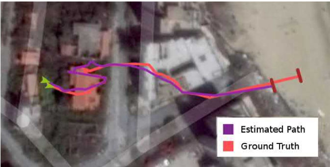
FIGURE 7.25 The ground-truth path of the UAV and the estimated path visualized on a map using their GPS coordinates using registration by shape matching in Famagusta.
