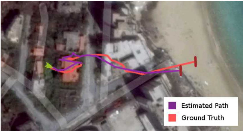
FIGURE 7.19 The actual path of the UAV and the estimated one visualized on a map using their GPS coordinates for the Famagusta Sequence.
